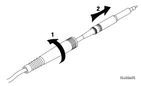
The cable strain relief may be unscrewed from the probe and slid back on the cable when using two or more probes in close proximity. When using the probe without the retractable hook tip, the barrel insulator (supplied accessory) should be used to cover the tip ground shield to prevent the hazard of shorting when probing the circuit. The barrel insulator, may be unscrewed and removed to accommodate tight probing situations.
